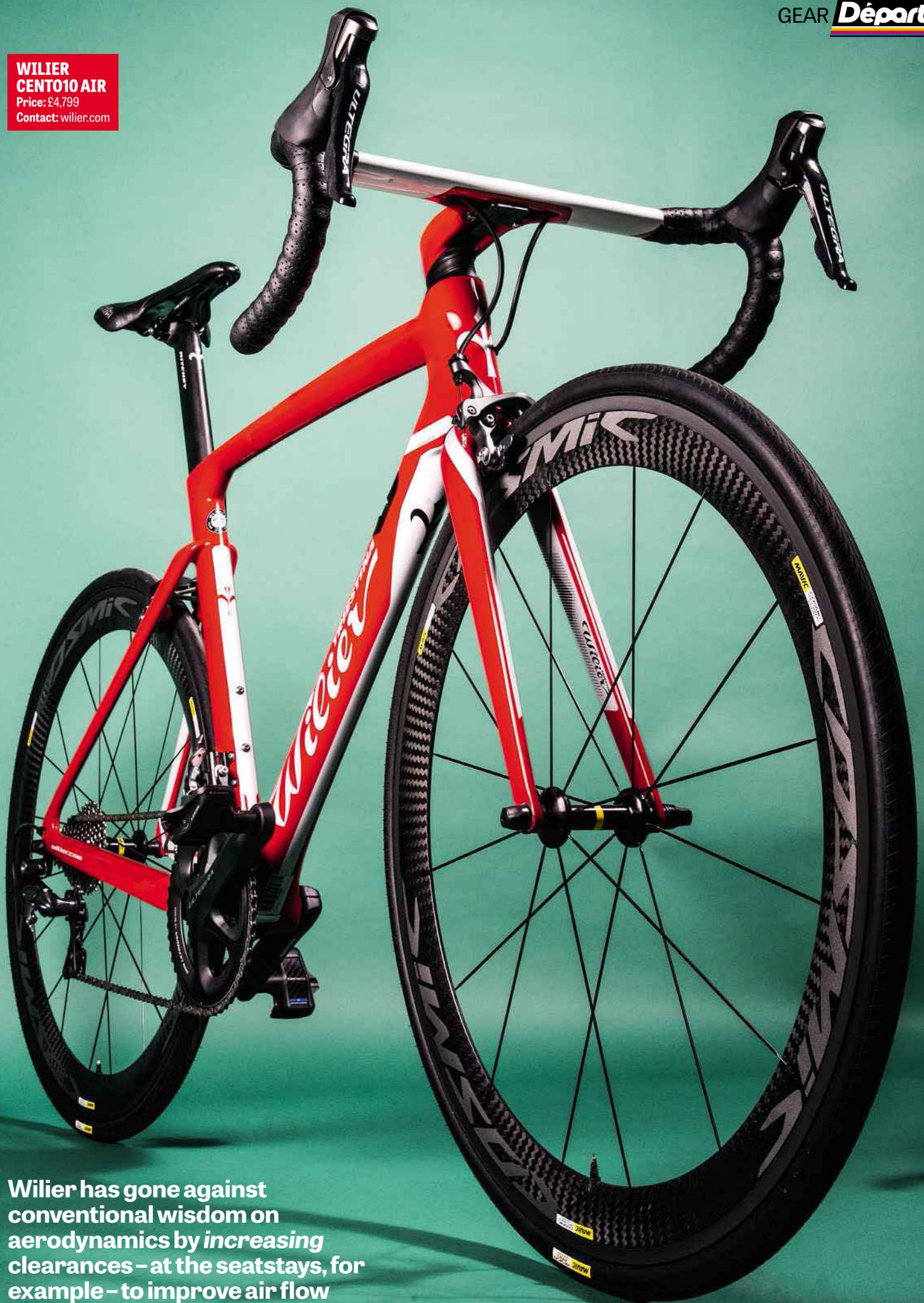
Wilier has gone against conventional wisdom on aerodynamics by *increasing* clearances – at the seatstays, for example – to improve air flow
