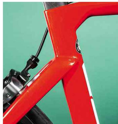
predecessor the Cento1. This isn't thanks to some miraculous new wonder material, but has been achieved simply by refining the lay-up of the carbon, working out which areas need less material and how to arrange the fibres to maximise strength. The result is a frame that's notably stiff and responsive but flies uphill as well as on the flat.
